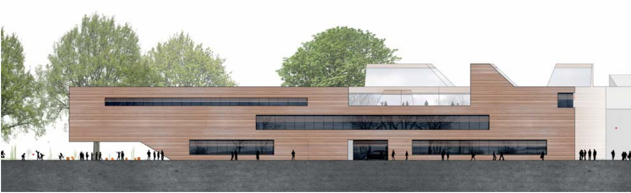
South elevation: larch-wood cladding and solar chimneys
