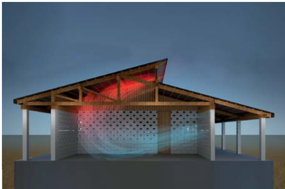
Natural ventilation system
